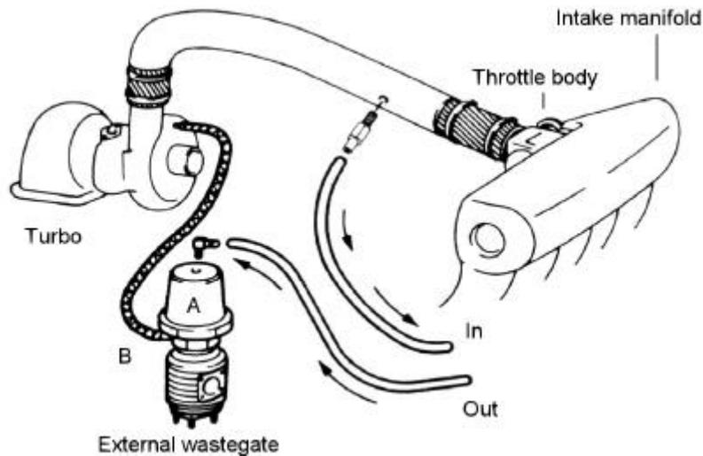
**IMPORTANT:** Compressor pressure must be between turbo and the throttle body.
