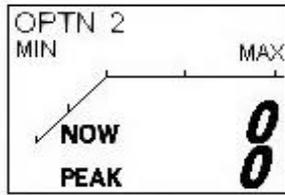
\* OPTN 2 is not used if Power Meter is not connected.
