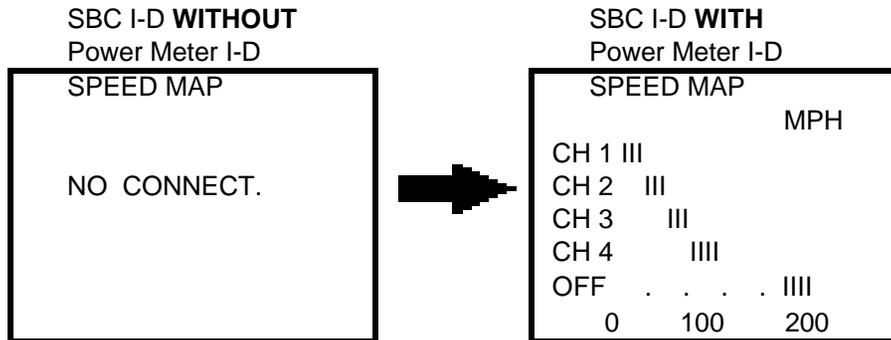
**Note:** For Speed Map to display MPH settings, you must change SBC I-D Unit setting to PSI.
